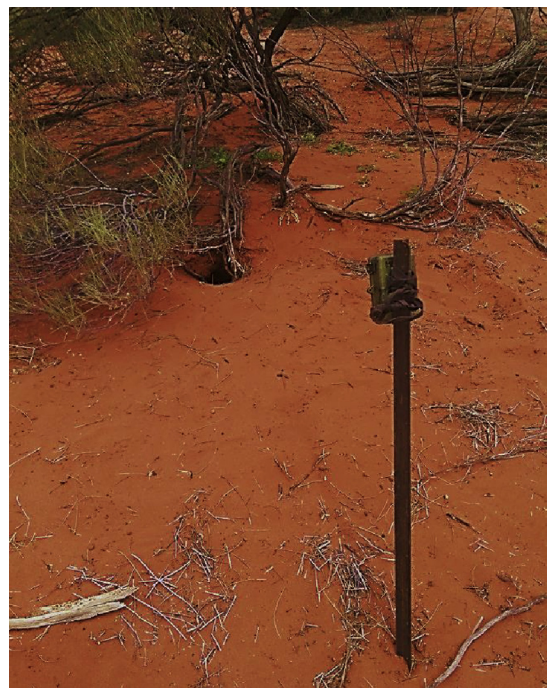
Figure 1. Experimental set-up for the bilby predator odour discrimination study. The photo shows the infrared motion sensor video camera mounted on a metal post outside the burrow entrance of a radiotracked bilby.
